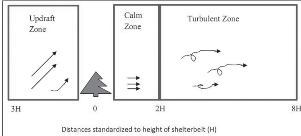
**Figure 1.** Diagram of the effect of shelterbelts on wind flow patterns around them (length of arrows reflecting relative wind velocity and distance from the shelterbelt is relative to the shelterbelt's height).
