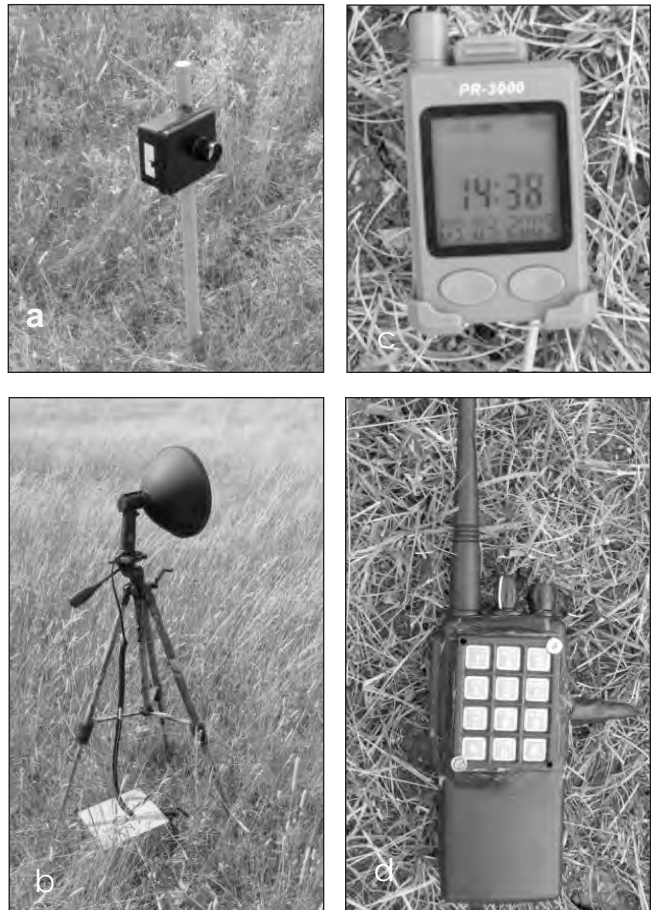
Figure 1. (a) Infrared motion detector (upper left); (b) receiver (grey box) and spotlight (lower left); (c) portable receiver, triggered by IR detector, indicating presence of animal on kill-site (upper right); (d) radio transmitter to turn on spotlights (lower right).
