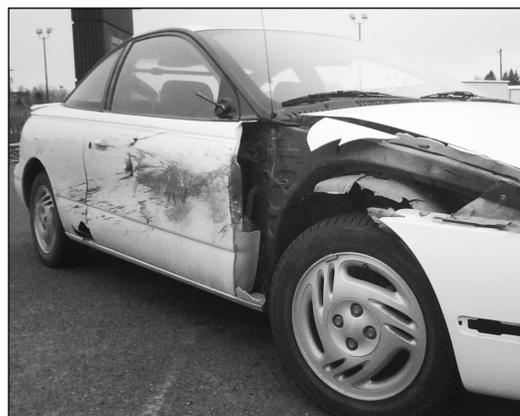
**Figure 1.** Damaged car after collision with deer.
