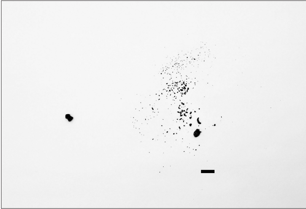
Figure 1. Lead bullets recovered from white-tailed deer ( Odocoileus virginianus ) from Litchfield County, Connecticut, USA, 2009–2011. An intact air rifle pellet (left), and a subset of the particles of a highly fragmented rifle bullet (right) are shown. Horizontal bar at lower right represents 1 cm.
